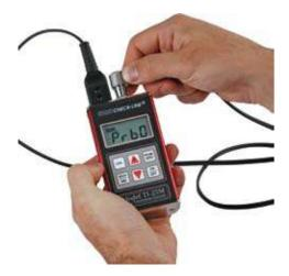
1. Connect probe and turn on gauge.
